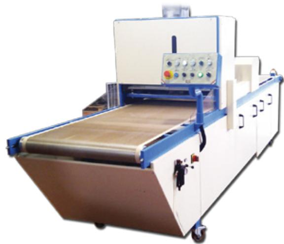
Innovative system for dusting transfer sheets, with new controls for flow and dispensed quantity. Equipped with a reverse cycle auger recirculation system for a work cycle without halts.
